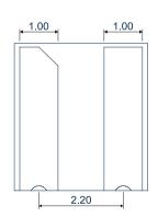
dimensions in mm, mechanical tolerance  $\pm 0.15$  mm unless otherwise noted
