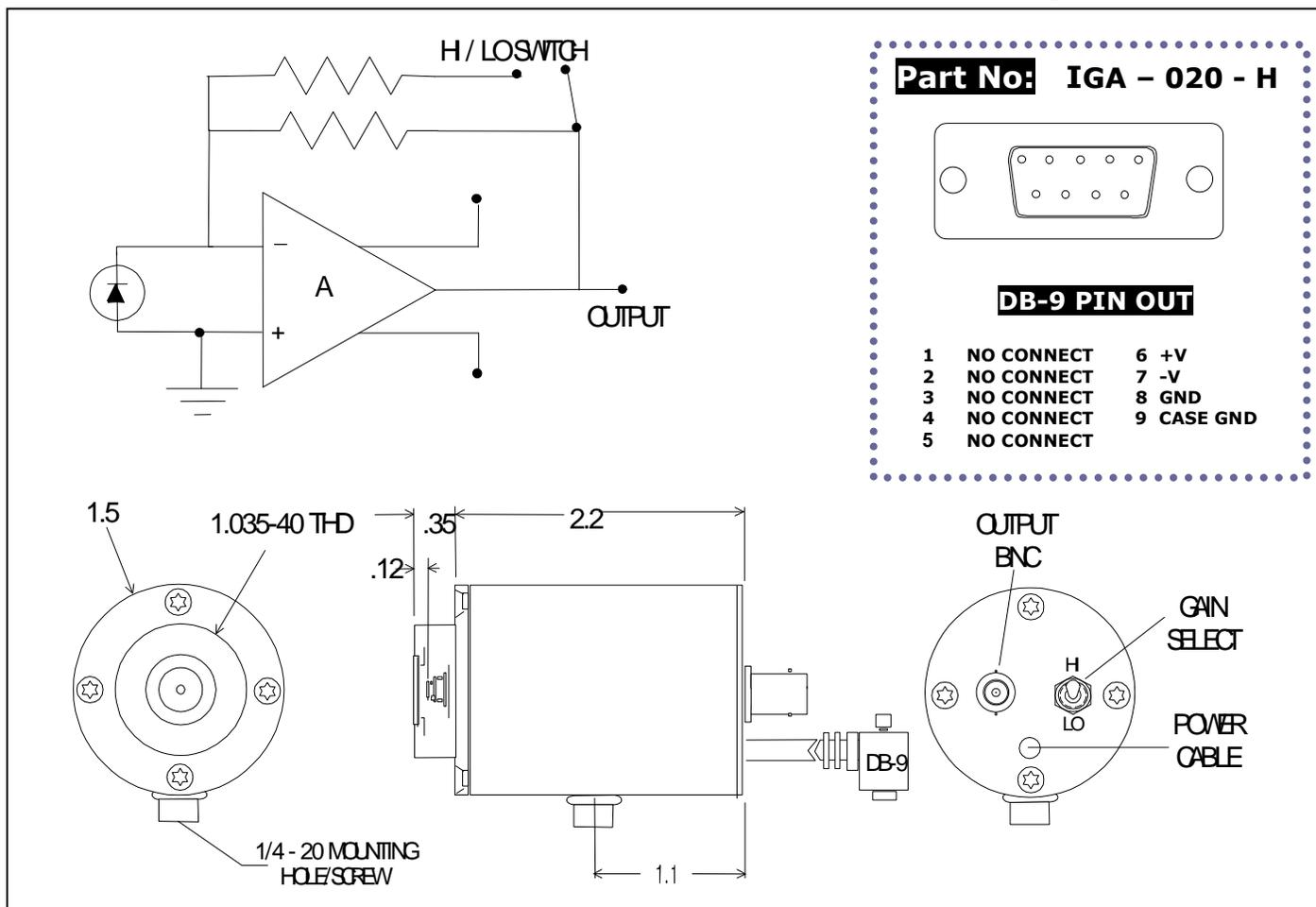
**Application Note** This unit is a high performance photodiode/receiver operated at ambient temperature with a dual gain FET input transimpedance amplifier. The output voltage is proportional to the input signal current:  $V_{out} = I_{signal} \cdot R_f$ . The PD/AMP is a DC coupled dual gain system. Care should be taken in shielding the unit from stray light during operation to prevent saturation of the amplifier (and potential failure).
