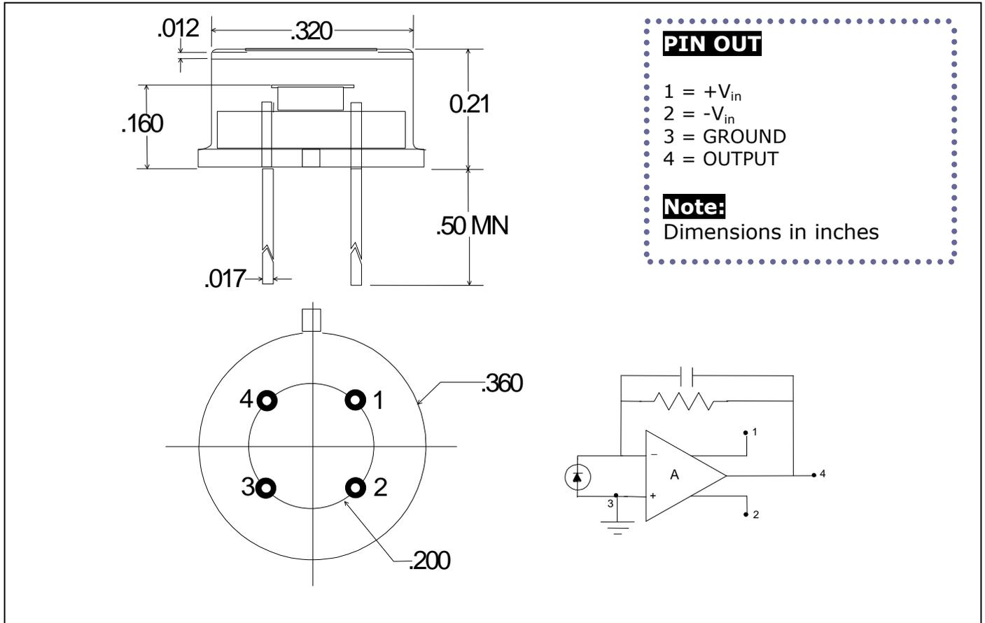
**Application Note** The preamplifier portion of this receiver is a transimpedance current to voltage converter. Its output voltage is proportional to the input signal current:
