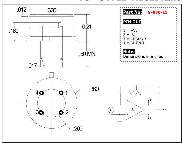
The preamplifier portion of this receiver is a transimpedence current to voltage converter. Its output voltage is proportional to the input signal current:
