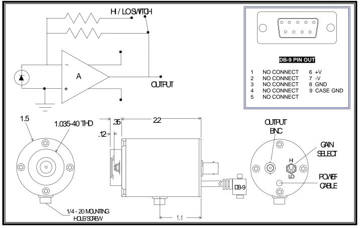
**Application** Note This unit is a high performance photodiode/receiver operated with at ambient temperature with a dual gain FET input transimpedence amplifier. The output voltage is proportional to the input signal current:  $V_{out} = I_{signal}$   $R_{f}$ .
