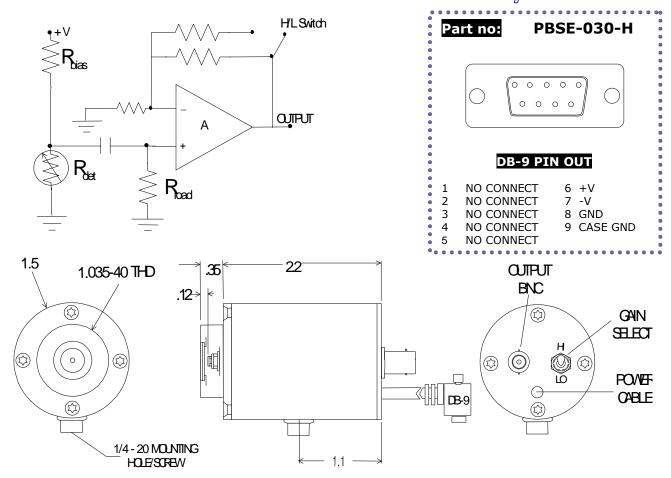
This unit is a high performance photoconductor/receiver operated at ambient temperature with a dual gain voltage amplifier. The detector's bias voltage is linked to the amplifier power supply and no additional biasing is necessary. The PC/AMP is an AC coupled dual gain detector system requiring a modulated input signal for operation.
